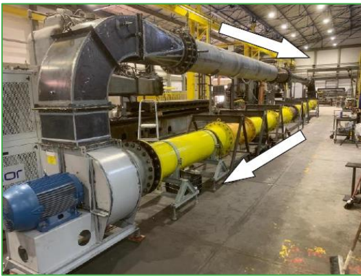
Fig 5. Front view of the circuit with the fan on the left. Source: IPT.
