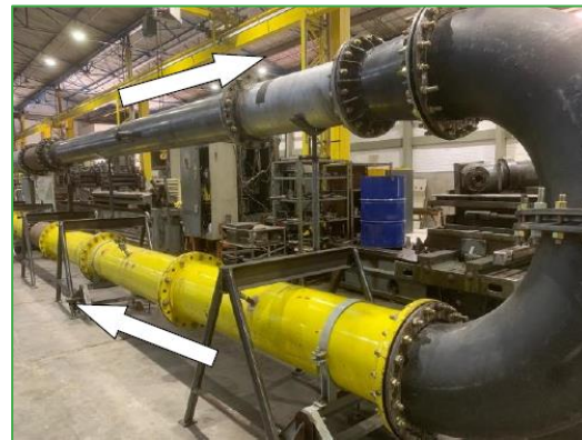
Fig 6. Rear view of the circuit showing the curve for fluid return to the fan. Source: IPT.
